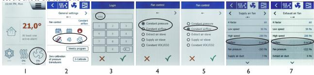
FAN SETPOINT high (set desired flow for running high) FAN SETPOINT low (set desired flow for running low)
